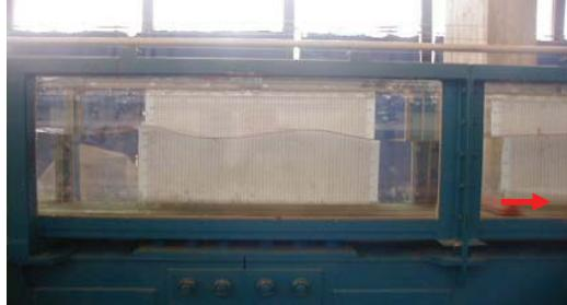
Fig. 11 Free-surface standing gravity waves
