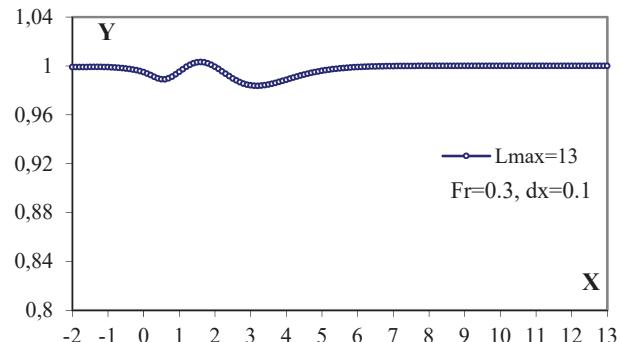
Fig. 6 Computed free-surface ( $F<1$ ,  $L_{max}=13$ )
