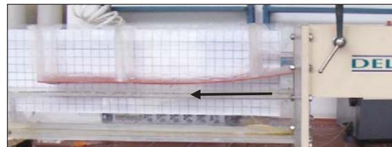
Fig. 13 Nozzle upstream for a supercritical regime
