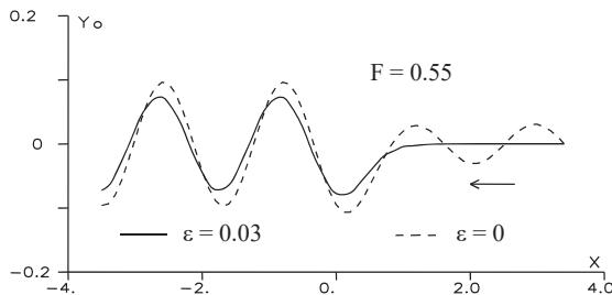
Fig. 7 The influence of the artificial viscosity  $\epsilon$
