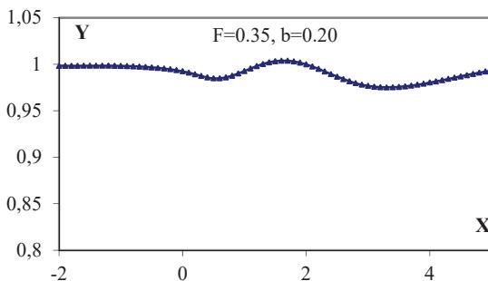
Fig. 5 Computed free-surface ( $F<1$ ,  $L_{max}=5$ )
