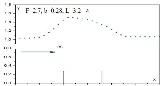
Fig. 14 Supercritical regime over a step
