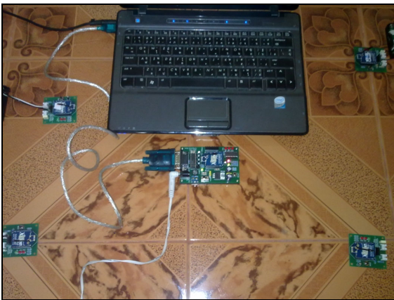
Fig. 4 Equipment used in the experiment: the referencing nodes and the object node
