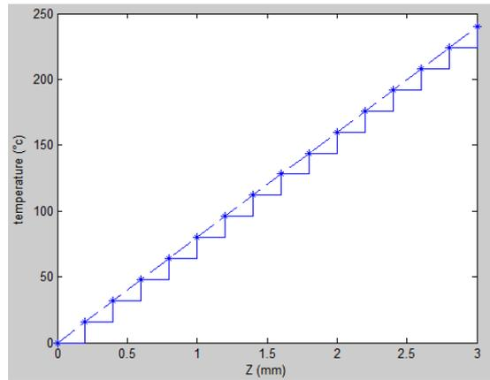
Fig. 4 (a) Non-uniform temperature applied on FBG
