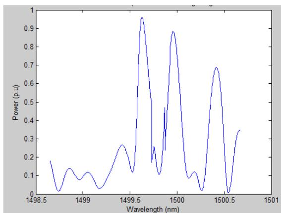
Fig. 5 (b) Shift of reflectivity spectrum under non-uniform strain
