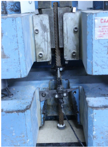
Fig. 1 UTM performing the pull-out test
