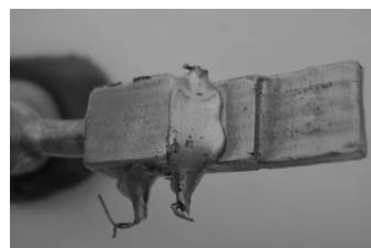
Fig. 8 The thermocouples were mounted in a stepped wedge to detect temperature during casting and cooling
