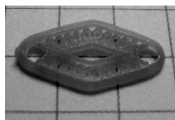
Fig. 4 The wax pattern of 'leaf-like' filigree object
