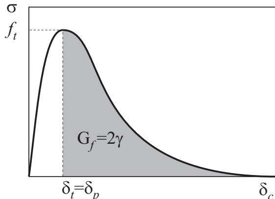
Fig. 4 Strain softening stress-strain and stress-displacement curves
