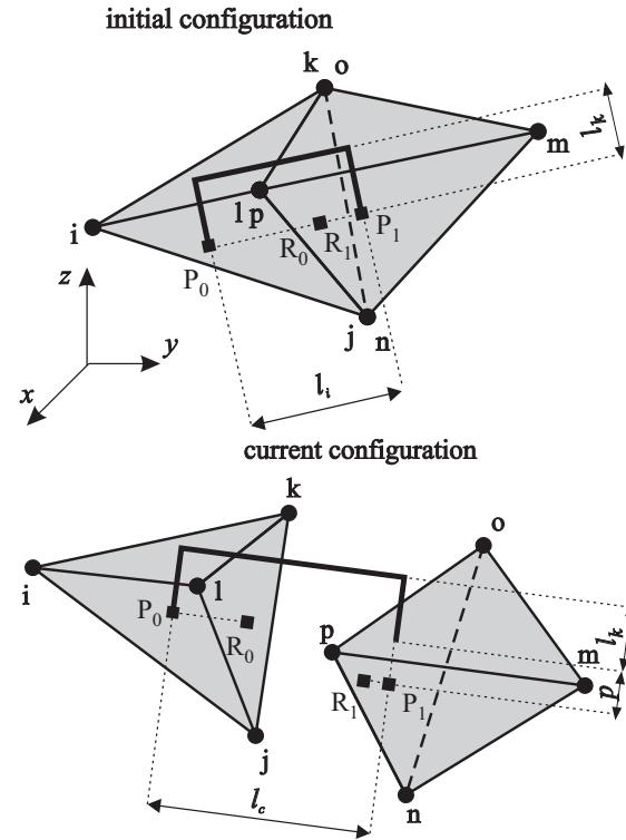
Fig. 7 Steel clamp in initial and current configuration.
