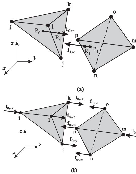
Fig. 9 Steel clamp: (a) force in steel clamp; (b) equivalent nodal forces
