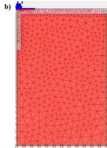
Fig. 3 Axisymmetrical numerical model in dynamic analysis, (a) Harmonic load on the surface, (b) mesh sizes in dynamic analysis
