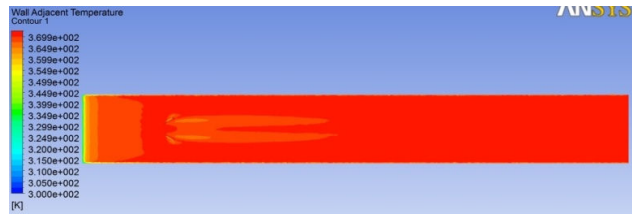
Fig. 13 Contours of wall adjacent temperature at Re 1200
