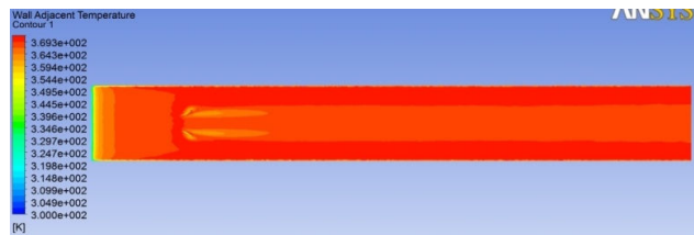
Fig. 15 Contours of wall adjacent temperature at Re 2000
