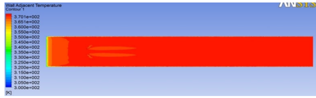
Fig. 12 Contours of wall adjacent temperature at Re 800
