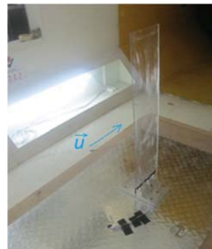
Fig. 2 Experimental setup for PC plate structure in Wind tunnel, Courtesy of Ankara Rüzgar Tüneli (ART)
