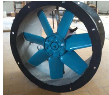
Fig. 3 Complete geometry of the counter-rotating rotor made
