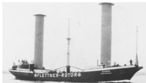
Fig. 1 Buckau - The first Flettner rotor ship [17]
