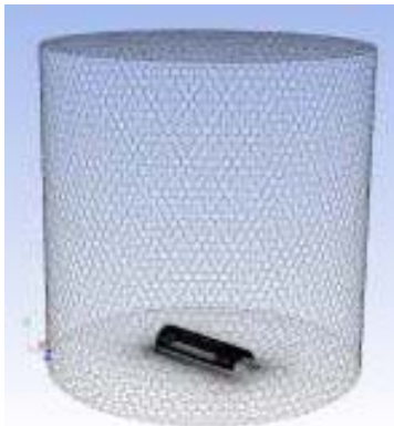
Fig. 8 Main geometrical features of the adopted grid inside the cylindrical sub-domain enclosing the building structure
