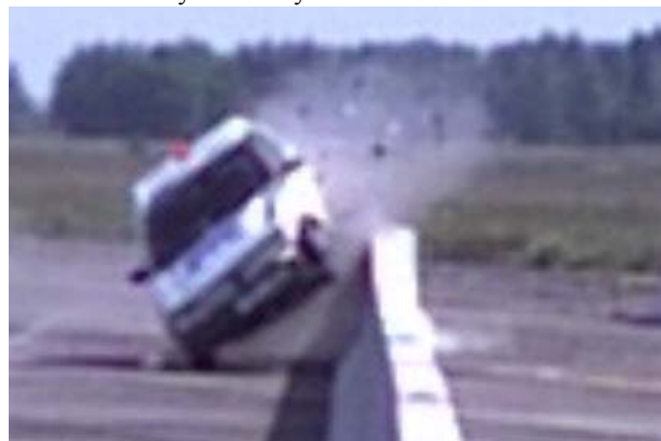
Fig. 4 Impact of light motorcar, speed of impact 105 km.h -1
