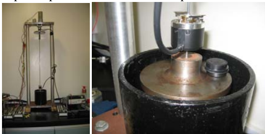
Fig. 1 Laboratory experimental drillstring set up and mass unbalance on lower rotor
