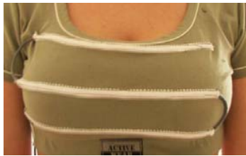
Fig. 7 Real photo of knitted shirt with piezofibers sensor in sensory shirt
