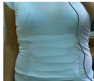
Fig. 4 Knitted shirt with optical fiber sensor
