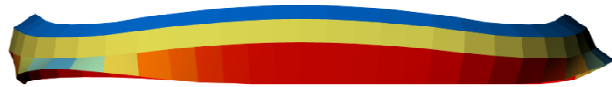
Fig. 8 Elevation – Visualisation of membrane slopes – Snow applies on blue panels (slope is less than 30°)
