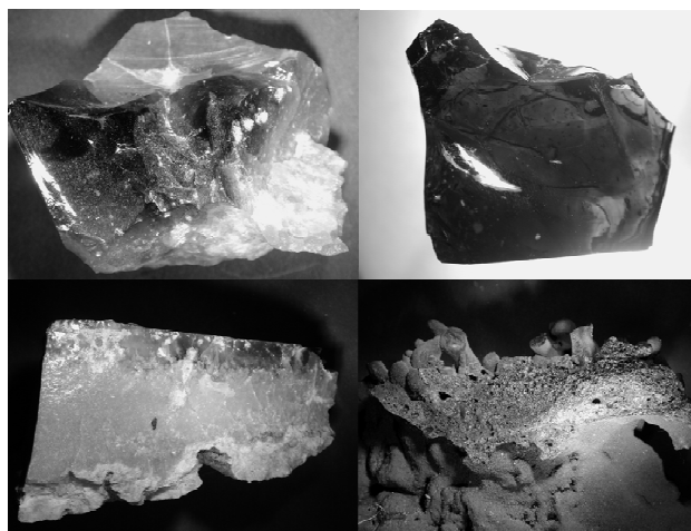
Fig. 1 Glass (upper) and partially crystalline (lower) deposits from a flamer part of the boilers that burned wheat straw (upper left), barley straw (upper right), rape straw (lower left), and brown wooden chips from pine loppings contaminated with soil
