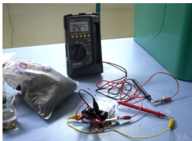
Fig. 3 Three series of compacted vermicompost produce 4.25V
