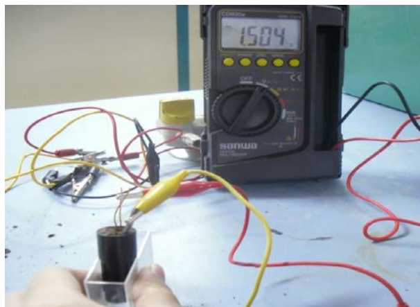
Fig. 2 One series of compacted vermicompost produces 1.504V
