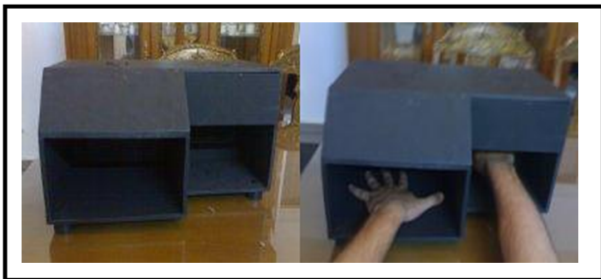
Fig. 1. Multimodal Biometric Prototype acquisition: the left compartment is for HG and FP and the right one is for the HV
