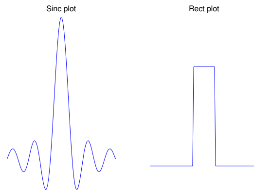
Fig. 8. Figure showing data in time domain and frequency domain (a) Sinc plot in frequency domain (b) Rect plot in time domain
