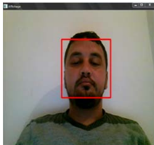
Fig. 1 Face detection by the Haar descriptor
