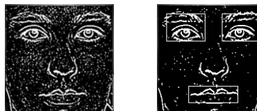
Fig. 2. Left: Edge detection results for the 7x7 laplacian of gaussian filter. Right: Edge detection results for the 7x7 laplacian of gaussian filter and the 3x3 medium filter
