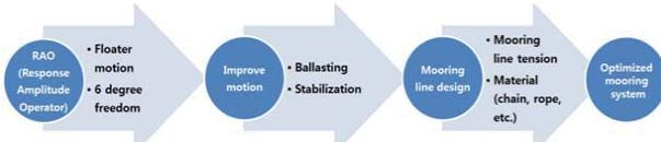
Fig. 2 Simplified procedure for mooring system design
