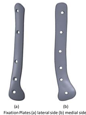
Fig. 3 Customized implant designed for fractured bone
