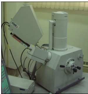
Fig. 3 SEM for studying built-up edge
