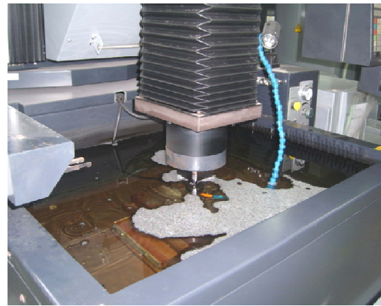
(a) EDM at machining state.
