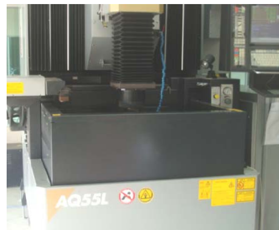
(b) EDM tank with electrode and workpiece.
