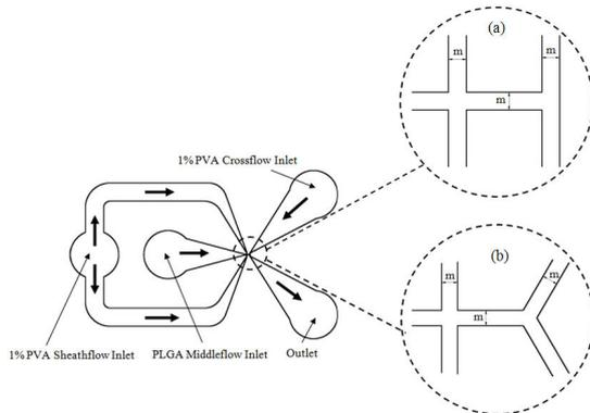
Fig 2 Schematic diagram of modified T-junction device: Channels are molded in PDMS. PLGA solutions with different concentrations are used: 1%, 5%, and 15%. *m*: channel width and height. (a) straight channel; (b) crooked channel
