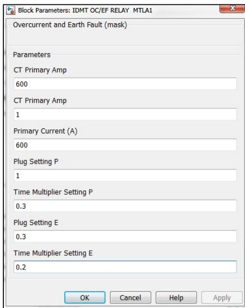
Fig. 5 Block parameters for phase and earth system
