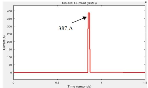
Fig. 20 RMS Earth Return Current for Case 13
