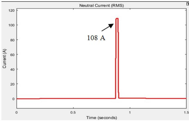
Fig. 15 RMS Earth Return Current for Case 9
