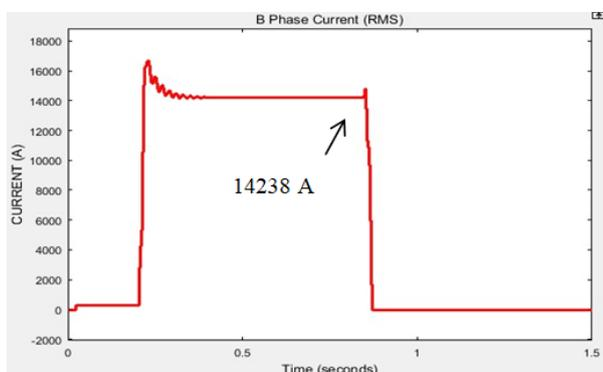
Fig. 19 RMS B phase Current for Case 13
