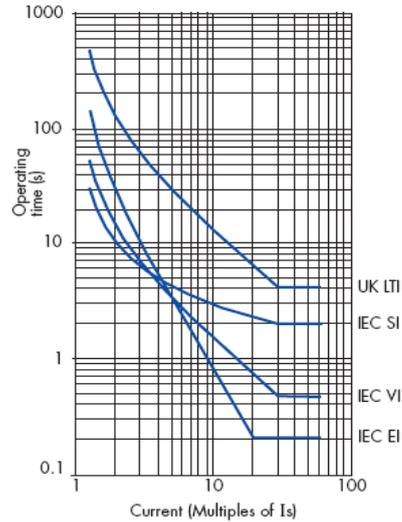
Fig. 1 Characteristics of Inverse Definite Minimum Time Curve
