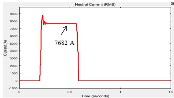
Fig. 11 RMS Earth Return Current for Case 5
