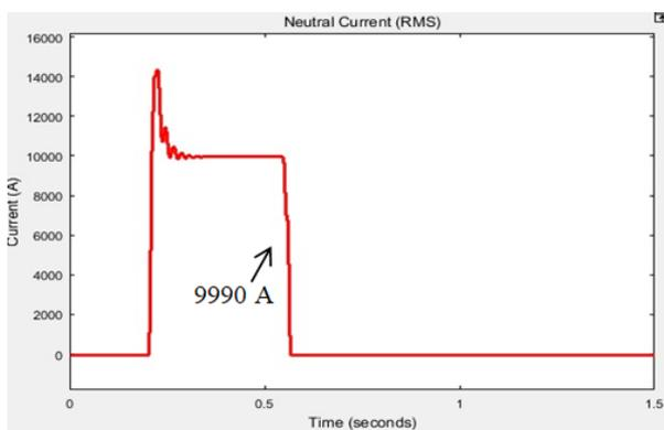
Fig. 7 RMS Earth Return Current for Case 1
