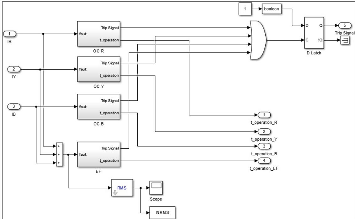
Fig. 4 Overcurrent and earth fault relay subsystem
