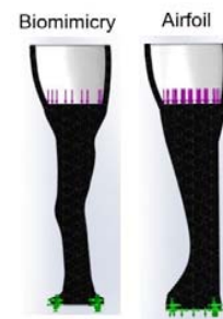
Fig. 13 Loading conditions for prosthesis
