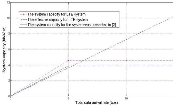
Fig. 2 Total data arrival rate against system capacity for the proposed LTE system and results of [2]. Also, the effective capacity for LTE system is presented
