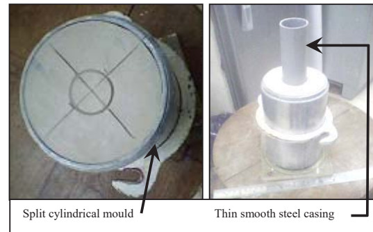
Fig. 3 Preparation of SCP in reconstituted clay specimen
