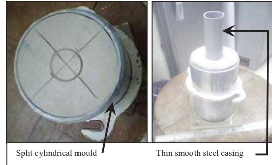
Fig. 3 Preparation of SCP in reconstituted clay specimen
