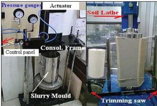
Fig. 2 Consolidation setup on the laboratory floor
