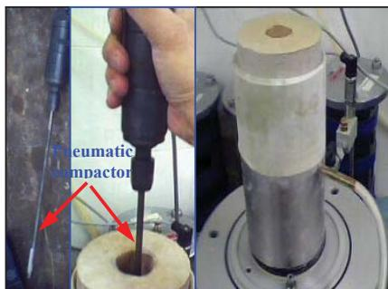
Fig. 4 Compaction of SCP in reconstituted clay specimen
