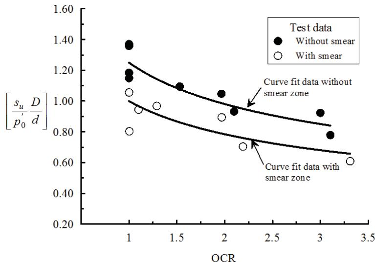
Fig. 12 Relationship between  $\left[ \frac{s_u}{P_0 \cdot d} \right]$  and OCR
