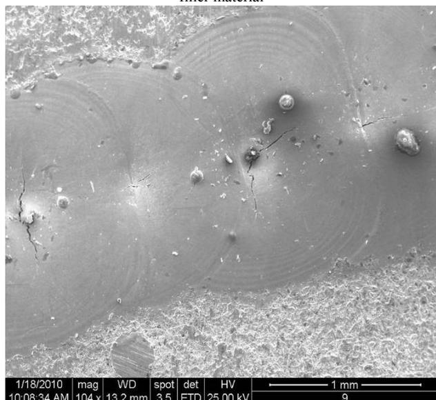
Fig. 6 Electron microscopically image of Heraenium NA alloy welded joints, without filler material: detail of short, radial cracks in the middle of the spot
