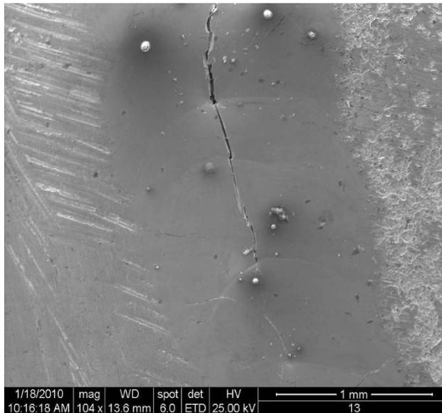
Fig. 7. Electron microscopically image of an SG Wirobond alloy welded without filler material: detail of a continuous longitudinal crack, and isolated oblique cracks in the welding rib.
