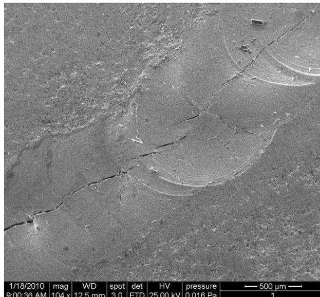
Fig. 3 Electron microscopically image of a Wiron 99 alloy welded without filler material: longitudinal discontinuous crack on the weld trajectory
