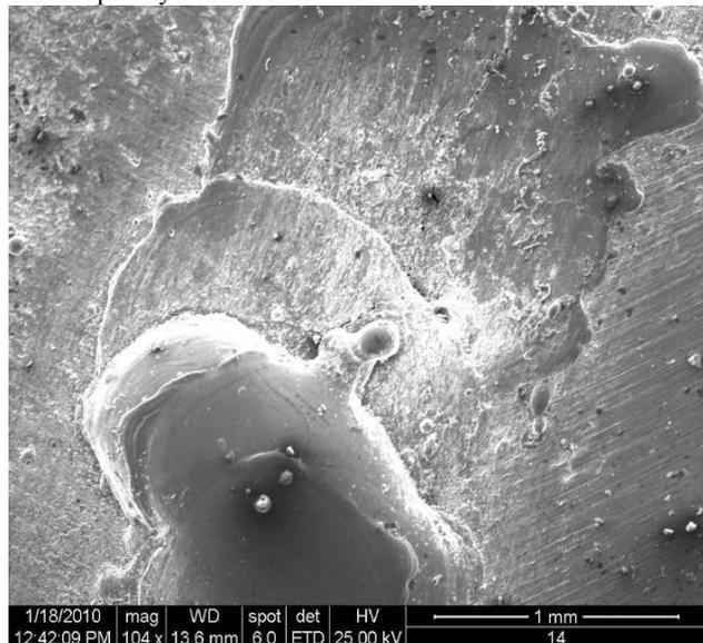
Fig. 5 Electron microscopically image of an SG Wirobond alloy welded with filler material: detail of ununiform distribution of the filler material
