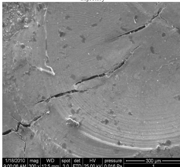
Fig. 4 Electron microscopically image of a Wiron 99 alloy welded without filler material: detail of an interrupted longitudinal crack on the weld trajectory
