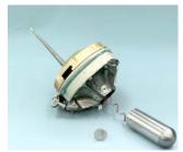
Fig. 1 Two body penetrator (DS2) [25]
