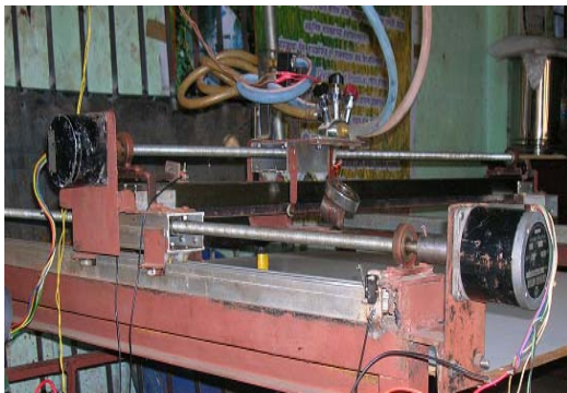
Fig. 5 Stepper motor mounted on the setup
