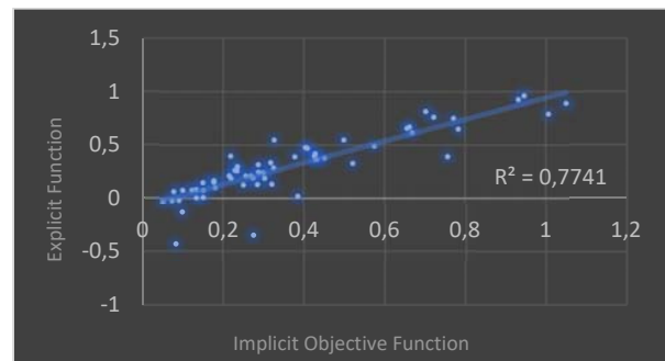
Fig. 9 Correlation between relative cost implicit and explicit objective functions for first case study with OMF
