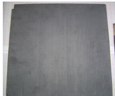
Fig. 2 Photograph of 3-D \text{C}_f/\text{SiC} composite laminate
