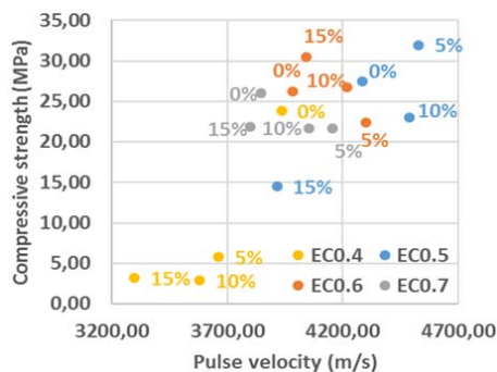
Fig. 4 UPV vs Compressive strengths for CH mixes
