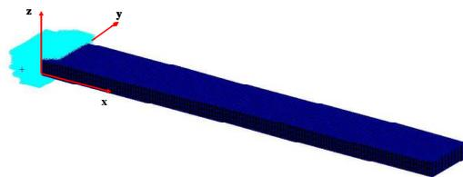
Fig. 7 The displacement boundary of a honeycomb sandwich plate
