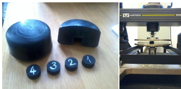
Fig. 1 The rubber bumper, the test pieces and the compression test
