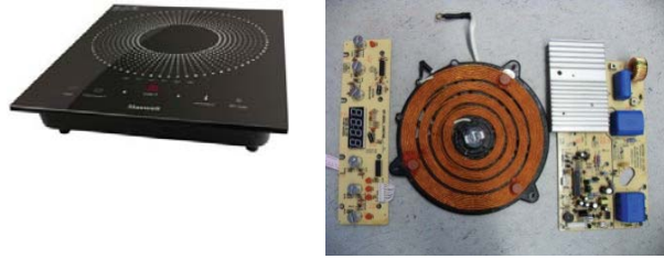
Fig. 12 Design of an induction cooker and its inductor
