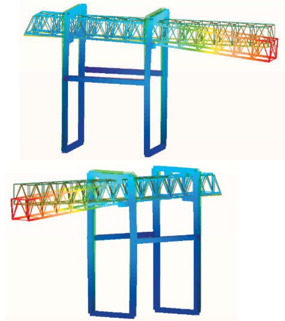
Fig. 4. Displacement of the crane with the pay load at sea side.
