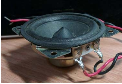
Fig. 1 The graph of moving-coil loudspeaker
