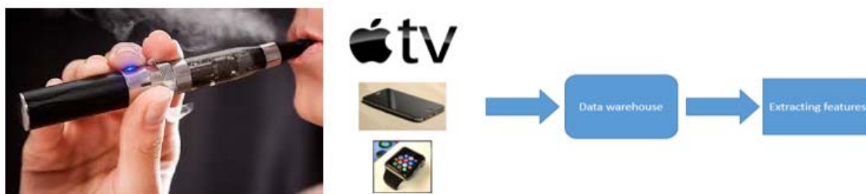
Fig. 2 Data collection system. The system contains an Extract Load Transform (ETL) that loads the data and integrates it into a data warehouse for later retrieval. The data warehouse contains several datamarts: a datamart for each sensor data
