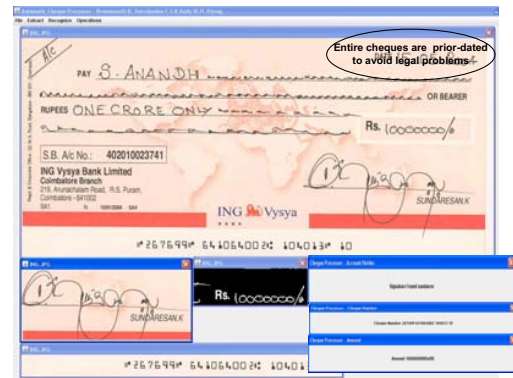
Fig. 14. A typical transaction of the proposed system by recognizing signature, cheque number and courtesy amount.
