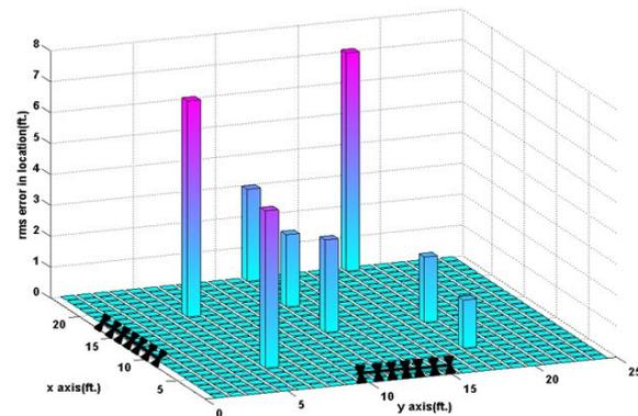
Fig. 3 Localization results of one unintended emitting RC device with far field bearing estimation technique
