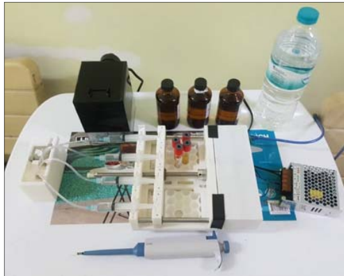
Fig. 3 RPHPLC Microfluidics System Hardware Setup
