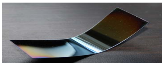
Fig. 9 Si foil of radius 252 mm shaped by hot plastic deformation
