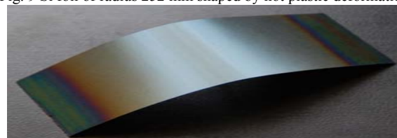
Fig. 10 Si foil of radius 398 mm shaped by hot plastic deformation
