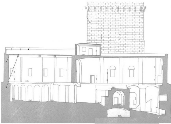
Fig. 17 Longitudinal section of the San Pancrazio Space after the soil removal
