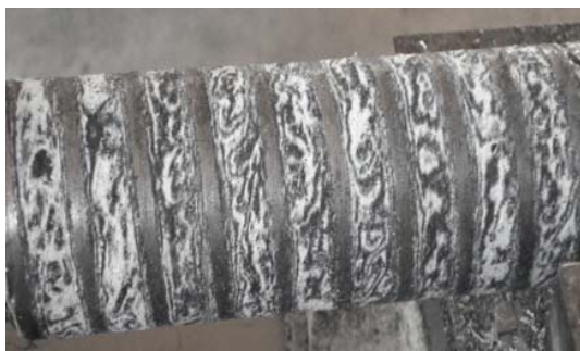
Fig. 3 Fibers wound on the mandrel
