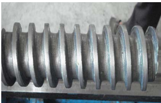
Fig. 2 Mandrel having the profile of the spring
