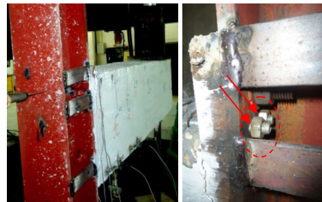
Fig. 12 Cracks in SP1 Beam and Splitting of the Steel Bars
